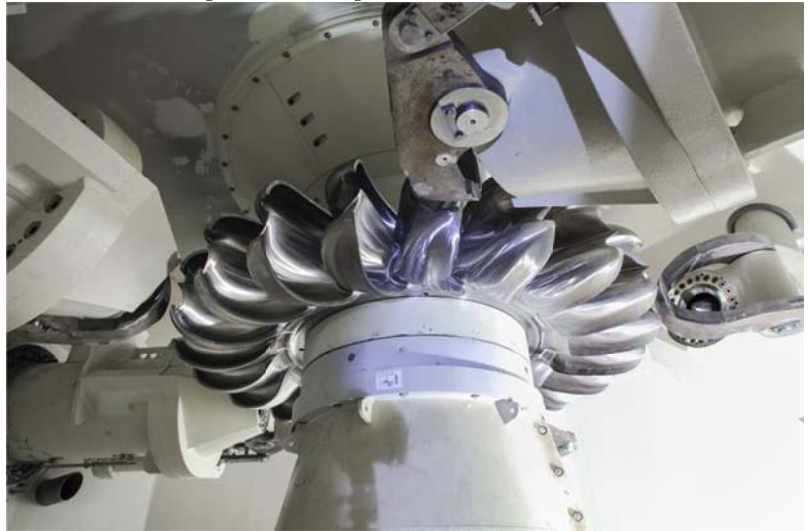
Figure 9. Main hydro-mechanical equipment. Pump (l), Pelton turbine (r).
